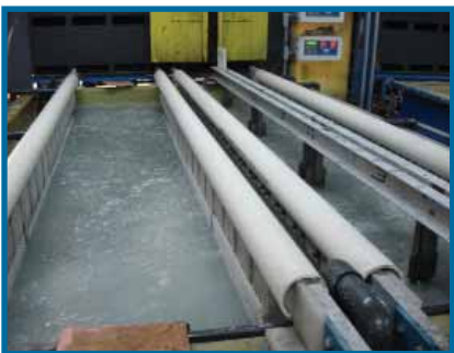
Nine-stage pretreatment line.
