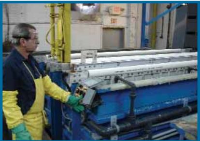
Experienced operators monitor each phase of the finishing process, including the triple-rinse stage.
